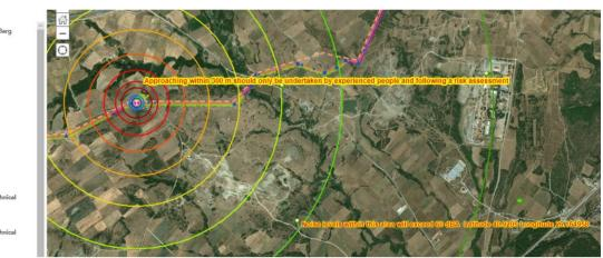
This example shows the noise contours if emergency venting is undertaken from a Block Valve. The contours have been developed from noise modelling and are included in the TAP GIS – this particular scenario is with a pipeline pressure of 5 bar (approximately the pressure during IOH)
